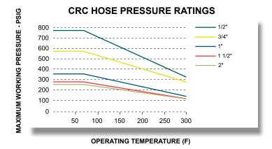
NOTE: For assemblies, pressure ratings of fittings may be less than for the hose.
