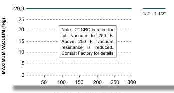
Note: Vacuum ratings are based on testing done on straight assemblies. Bent assemblies may have reduced vacuum resistance.
