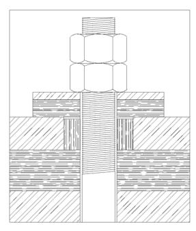
Fabreeka® has been used for many years for mounting heavy machinery where absorption of shock and isolation of transmitted vibration is desired. Fabreeka distributes the load properly; prevents cracking and flaking of concrete; eliminates the need for grout; prolongs the life of both machines and buildings. Fabreeka is scientifically constructed to give years of service under the most severe operating conditions.
