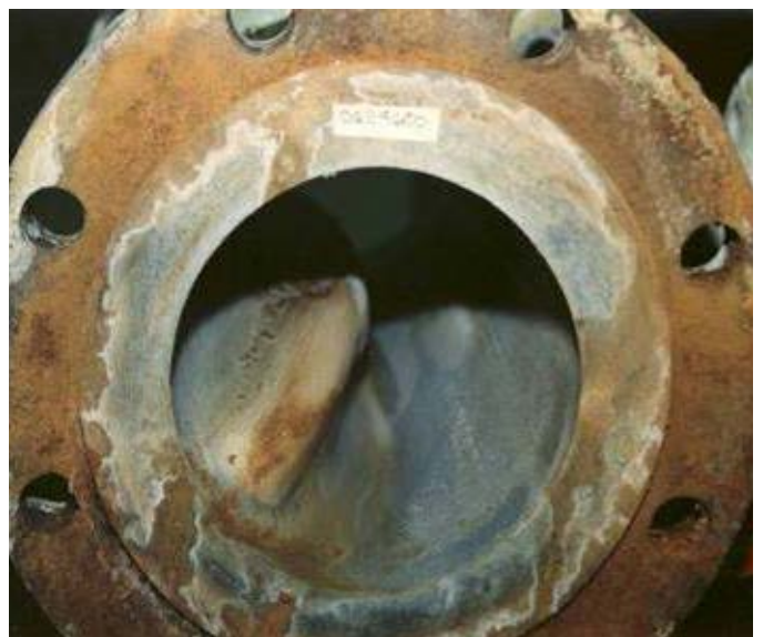
Single Lobe Liner Collapse
