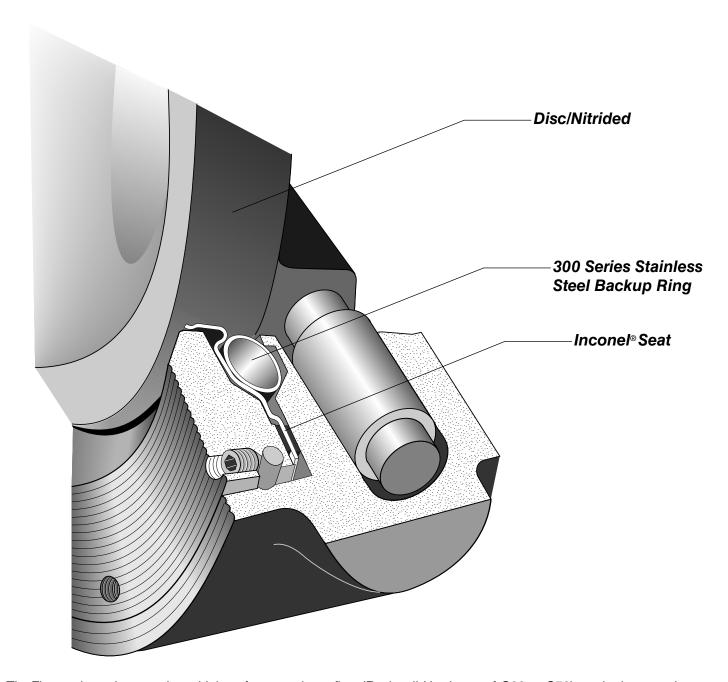
The Flowseal metal-to-metal seat high performance butterfly valve incorporates an Inconel® seat for higher tensile strength, a 300 series stainless steel back-up ring in the seat cavity for axial seat support, and a disc that is case hardened by nitriding.
