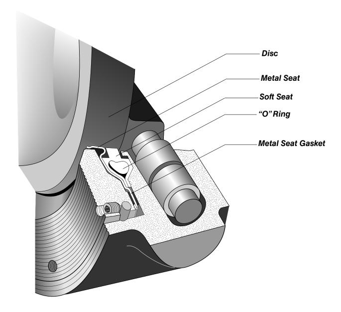
The Flowseal Fire-Flow™ high performance butterfly valve (HPBV) is a fire-safe, soft seat quarter-turn valve. The Fire-Flow™ design incorporates two patented seats which function together to seal off pipeline flow. In normal operation, the soft seat provides a bi-directional "bubble tight" shutoff (zero leakage); the metal seat provides bi-directional shutoff in the event of a fire, in conformance to industry fire-safe requirements.
